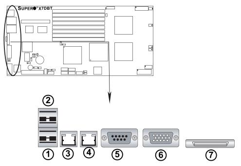
Figure 2-3. Back Panel I/O Port Locations and Definitions
